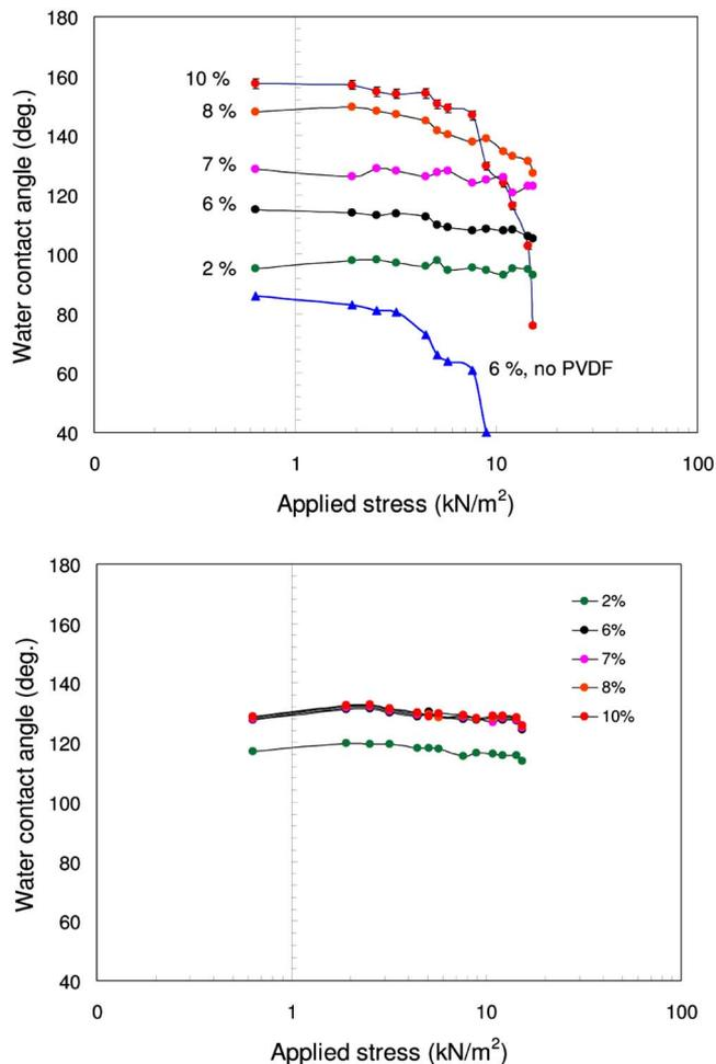
FIG. 3. (Color online) Sessile water contact angle variation as a function of applied tensile stress. (a) Coatings containing unmodified ZnO nanopowder. The reductions in contact angle were accompanied by flaking of coatings under mechanical stress. The coatings withstood 3–5 kN/m<sup>2</sup> depending on their composition. (b) Coatings containing functionalized ZnO. The contact angle is nearly insensitive to ZnO concentration beyond 6 wt %.
