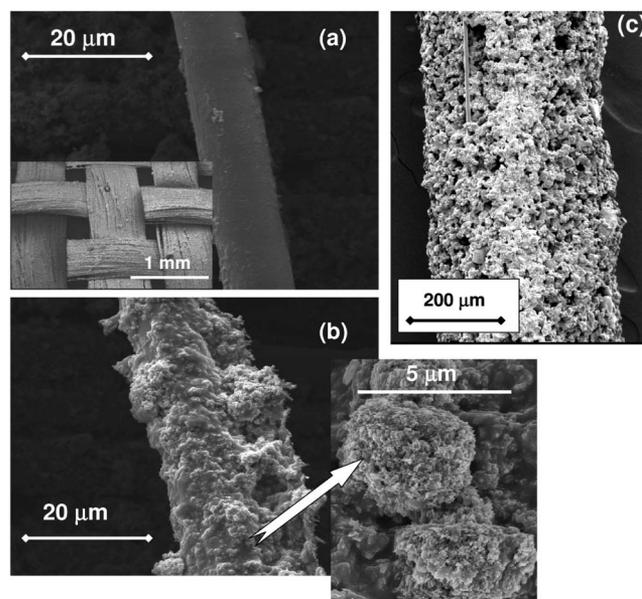
FIG. 2. SEM micrographs of (a) uncoated glass fiber of approximately 10  $\mu\text{m}$  in diameter. The inset shows the morphology of the coated glass-fiber yarn using dry ZnO nanopowder. (b) Coated glass fibers isolated from the fiberglass cloth. The magnified detail shows the surface micro-/nanoscale morphology of the coating. (c) A bundle of glass fibers with a microporous PVDF/CA/rosin coating filled with unmodified ZnO microparticles ( $\sim 5$   $\mu\text{m}$ , 8 wt %).
